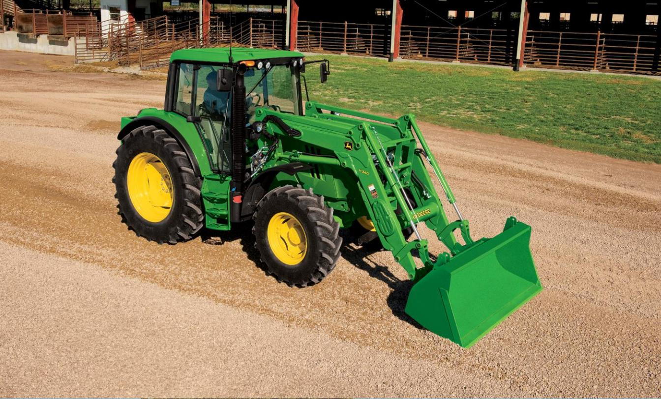
The transmissions on 6M Tractors are great for loader work. All cab tractor transmissions feature reversers. On the open operator station models, the PowrQuad transmission features a reverser. Just flip a lever on the left side of the steering wheel and you change directions. The transmission features oil-cooled clutches for longer life, and smooth direction changes.
