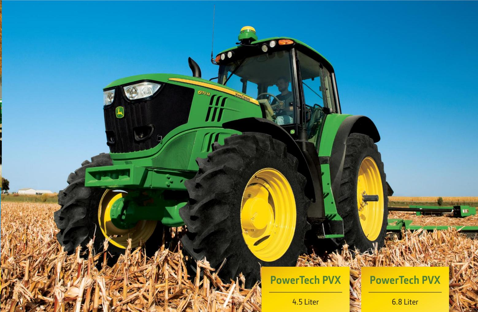
On all John Deere 6M Tractors you benefit from of a full-frame design. The engine, transmission and other components are supported by the steel frame, which resists the stresses of loader and hitch work. The full frame not only helps protect the engine and transmission, it makes access to components easier for faster routine maintenance and service.
